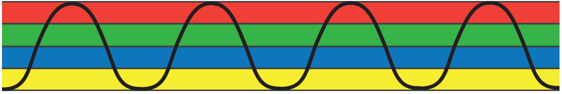
Figure 2.22: Graphical representation of amplitude gating. Here the pseudo sinusoidal signal represents the SS and the horizontal lines, colour coded differently, represent the amplitude gates that the data upon the SS would be binned into.
