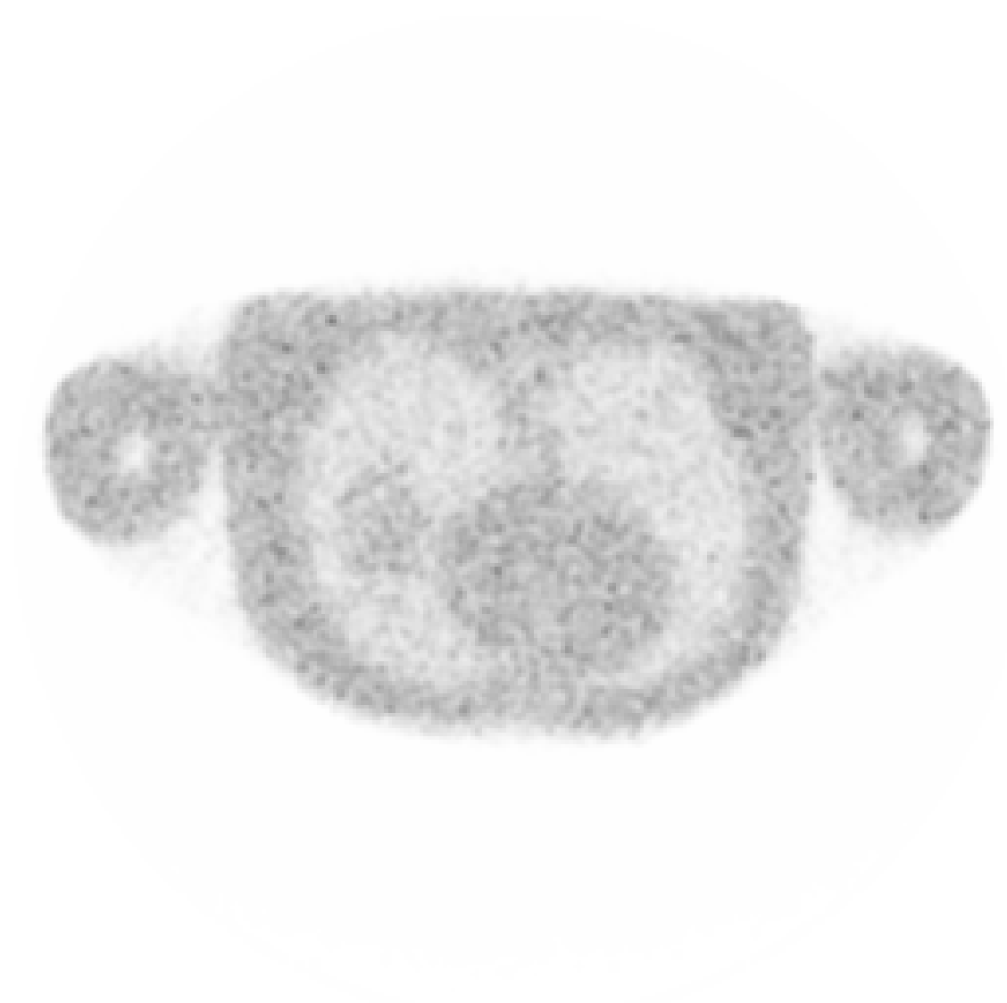
Figure 2.15: Example of a simulated AC Non-TOF Ordered Subset Expectation Maximisation (OSEM) reconstruction, with motion and noise, with no randoms or scatters, of the thorax with a spherical lesion in the lungs. Transverse view.
