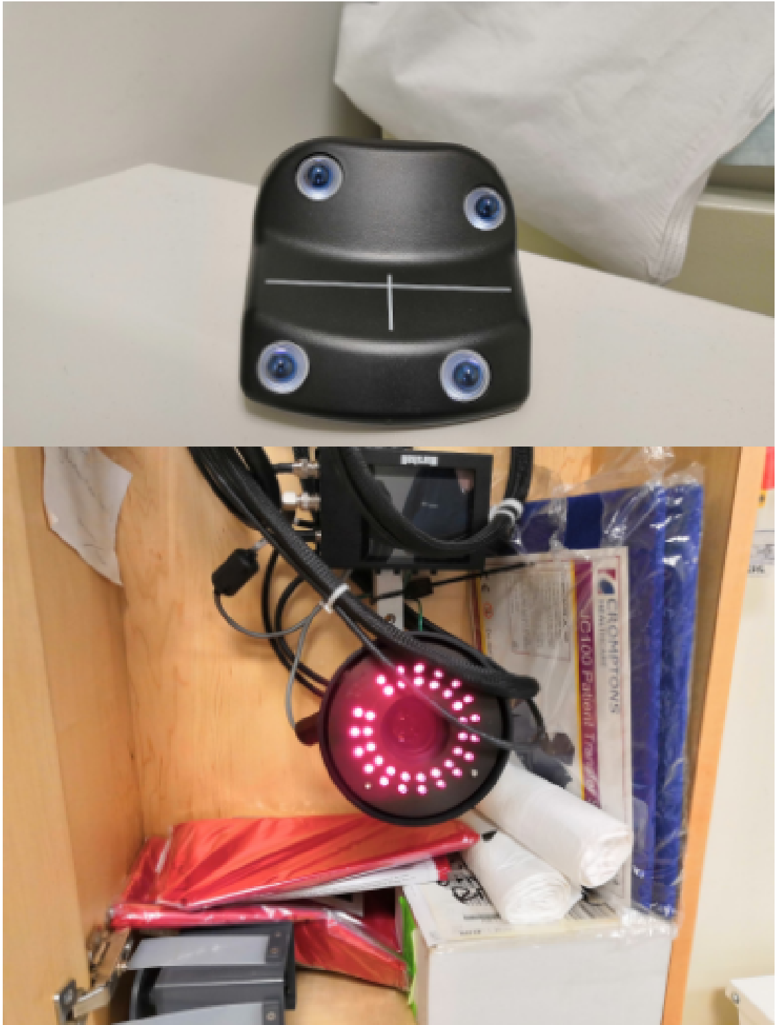
Figure 2.24: Photograph of the RPM. On the bottom of this figure is the infrared camera and infrared Light Emitting Diodes (LEDs) used to locate and track an infrared reflecting marker. On the top of this figure is the infrared reflecting marker which is placed onto the chest or stomach of the patient in order to track the respiratory amplitude of the patient. Four reflective points are used to track the marker in 3D.
