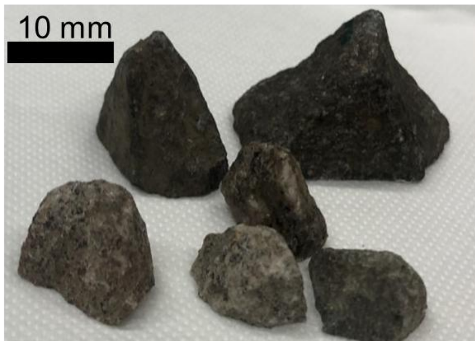
Figure 3.14 Washed used granite samples (from the UK) after cutting to the right size and after washing and cleaning.
