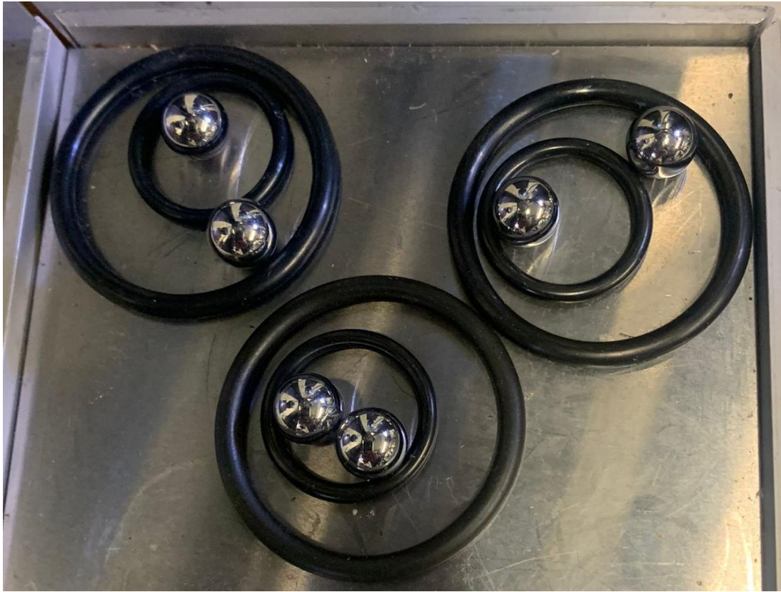
Figure 3.49 The 3-point bearing system to measure friction modified by the author and Dr Saurabh Singh.
