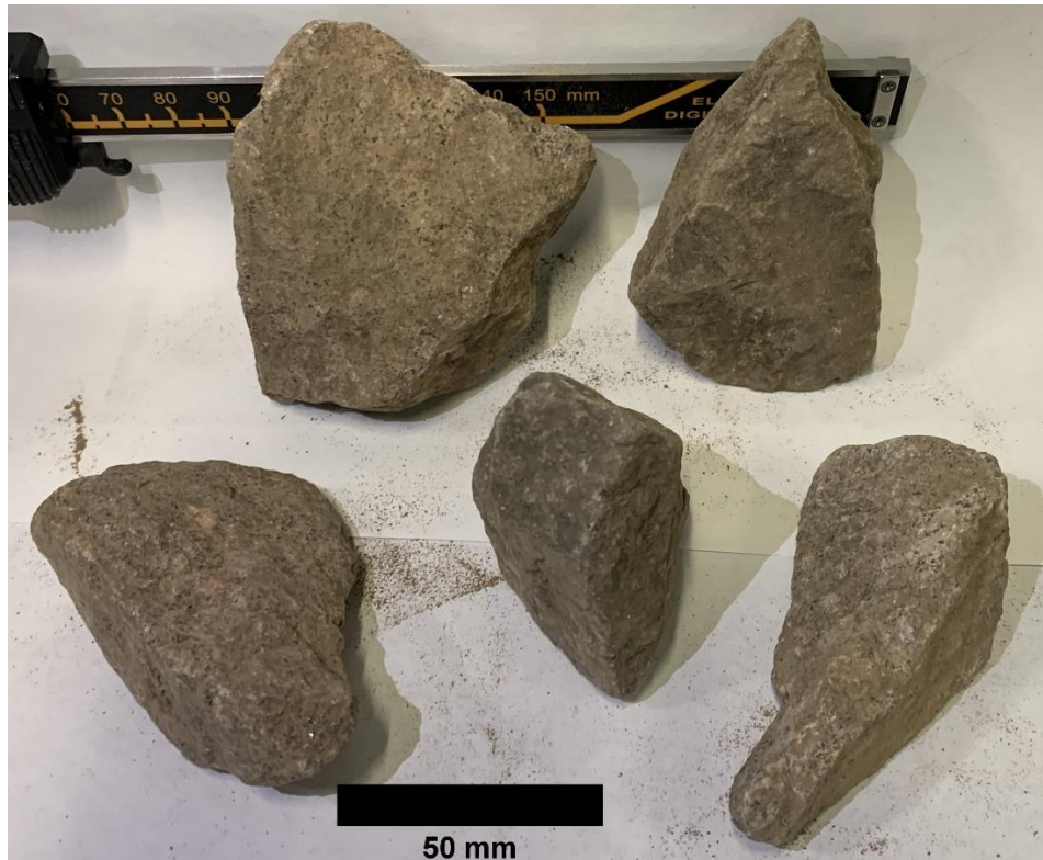
Figure 3.13 Used granite samples (from UK) selected for testing, shown in their natural state without any washing or cleaning.
