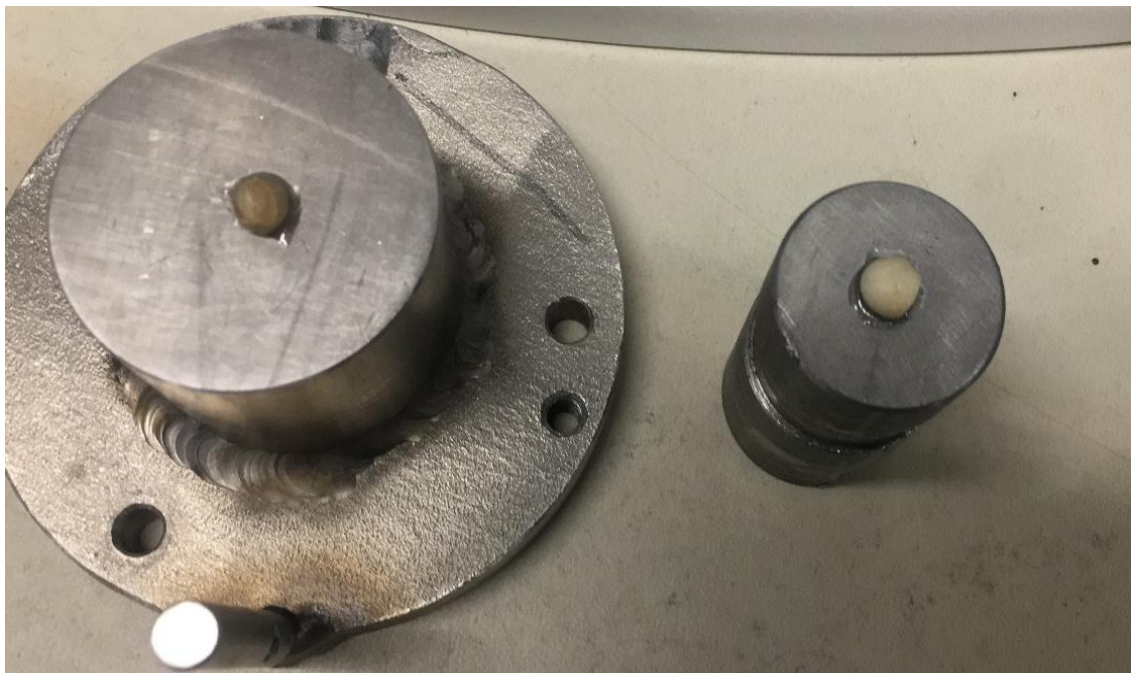
Figure 3.21 After the dead load is removed, the particle position is checked
