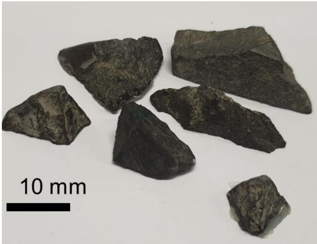
Figure 3.9 Australian basalt ballast particles are washed and dried before testing
