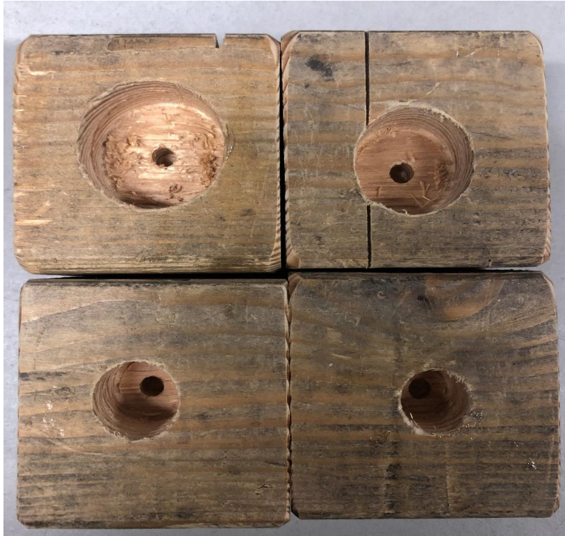
Figure 3.18 Custom-made protective caps for big particles (ballast).
