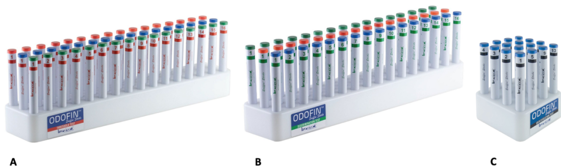
Figure 2.5. Sniffin' Sticks extended test including threshold (a), discrimination (b) and identification (c) tests.
