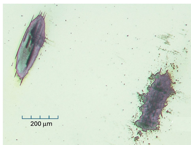
Fig. 5 Optical micrographs of laser burn marks. The rough-shaped burn was obtained through the Mylar window of the sample chamber, giving rise to optical speckles.
