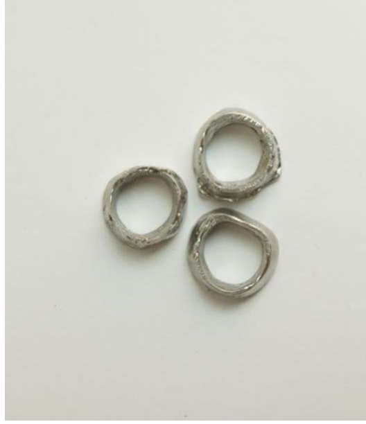
Figure 17: Three pewter rings made by casting pewter into hand formed clay. Copyright: Xan Xacobo Goetzee-Barral, 2023.
