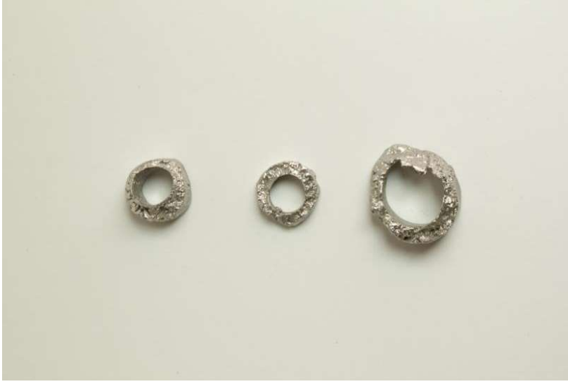
Figure 19: Pewter rings cast by implanting a stick into ground in my back garden to create the mould. Copyright: Xan Xacobo Goetzee-Barral, 2023.
