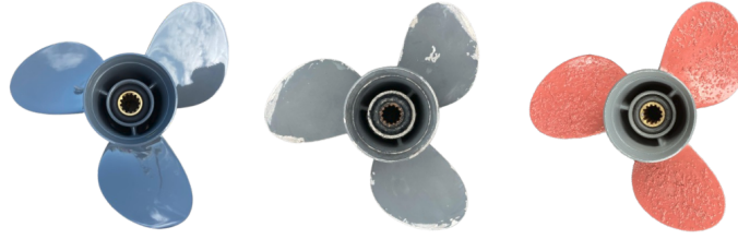
Figure 4: The clean, damaged and artificially roughened propellers.
