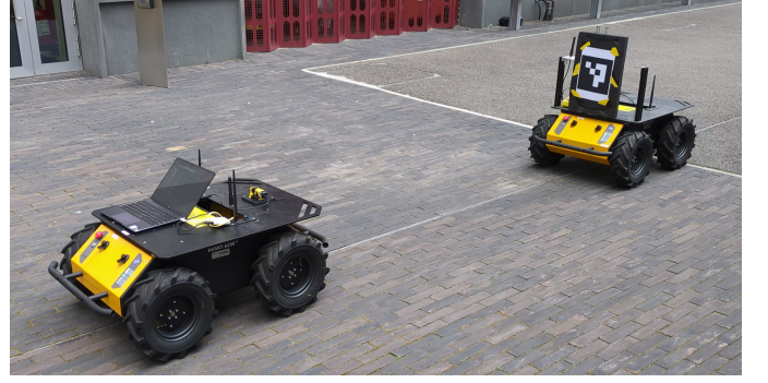
Fig. 7. Experimental setup involving two Husky A200 unmanned ground vehicles.
