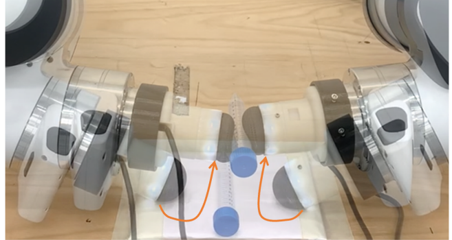
Fig. 1: Autonomous dexterous grasping with soft tactile sensors, including pre-grasp, press, roll-lift, and firm grasp.
