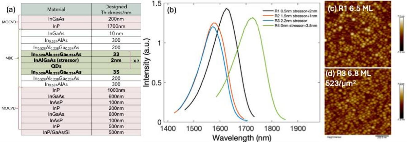
Fig. 1. (a) Schematic epitaxial structure of the InAs/InP QD laser on Si. (b) PL spectra of InAs/InP QDs with different capping layers. (c) and (d) AFM images of 6.5 ML and 6.8 ML InAs deposition, respectively, with the latter showing a high dot density of  $523/\mu\text{m}^2$ .
