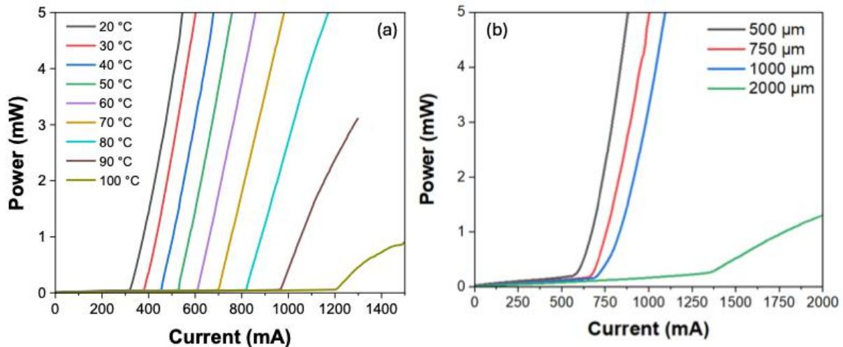
Fig. 2. (a) Temperature-dependent current versus power L-I curves under pulsed injection for  $2000\text{ }\mu\text{m} \times 5\text{ }\mu\text{m}$  cavity InAs/InP QD lasers on Si. (b) Current versus power L-I curves under pulsed injection for  $50\text{ }\mu\text{m}$  cavity width InAs/InP QD lasers on Si with varied cavity lengths from  $500\text{ }\mu\text{m}$  to  $2000\text{ }\mu\text{m}$ .
