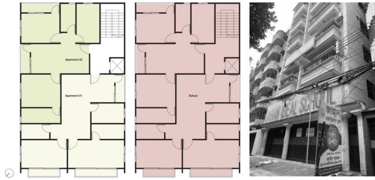
Figure 2. (left) Original (adopted by observation) two unit apartment plan: Approx. 1600sft total, (middle) Adapted layout for a primary school, (right) the exterior view of the typical apartment building front (Source: Author)
