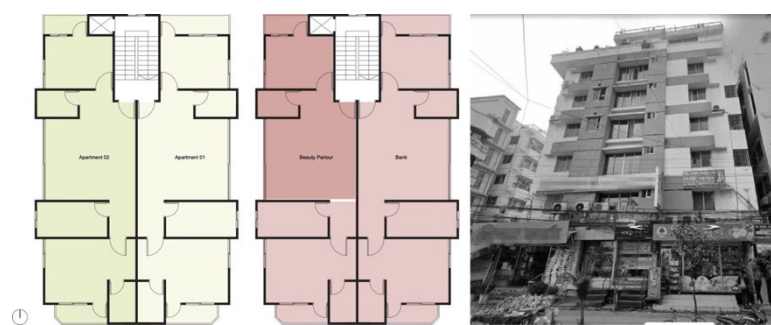
Figure 5. (left) Original (adopted by observation) two unit apartment plan ~1600sft, (middle) Adapted plan for a Beauty Parlour ~450sft and Bank ~1200sft, (right) the exterior view of the typical east view (Source: Author)
