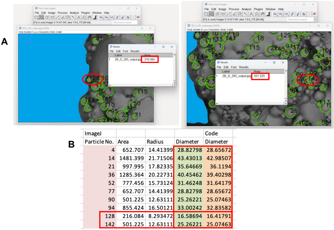
Figure 4.N: A) Examples using the circle tool in ImageJ to measure the specific particles. B) The areas measured for the 10 chosen particles were converted into diameters and compared with the measurements found by the code to check for concurrent values. Examples in (A) are indicated. These steps were applied to all cups counted and measured using the computerised method.
