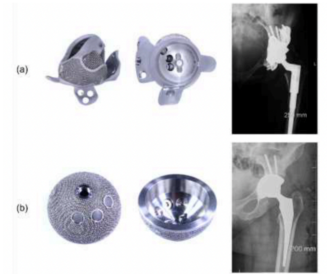
Figure 2.09: Outer (backside) and internal surface of (a) custom and (b) off-the-shelf 3D-printed acetabular implants. Antero-posterior (AP) plain radiographs are also shown.
