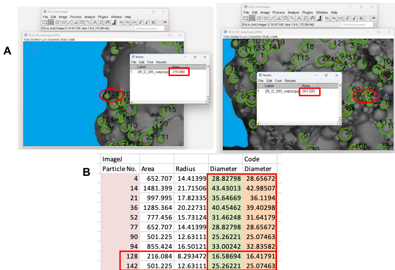
Figure 4.06: A) Examples using the circle tool in ImageJ to measure the specific particles. B) The areas measured for the 10 chosen particles were converted into diameters and compared with the measurements found by the code to check for concurrent values. Examples in (A) are indicated. These steps were applied to all cups counted and measured using the computerised method.
