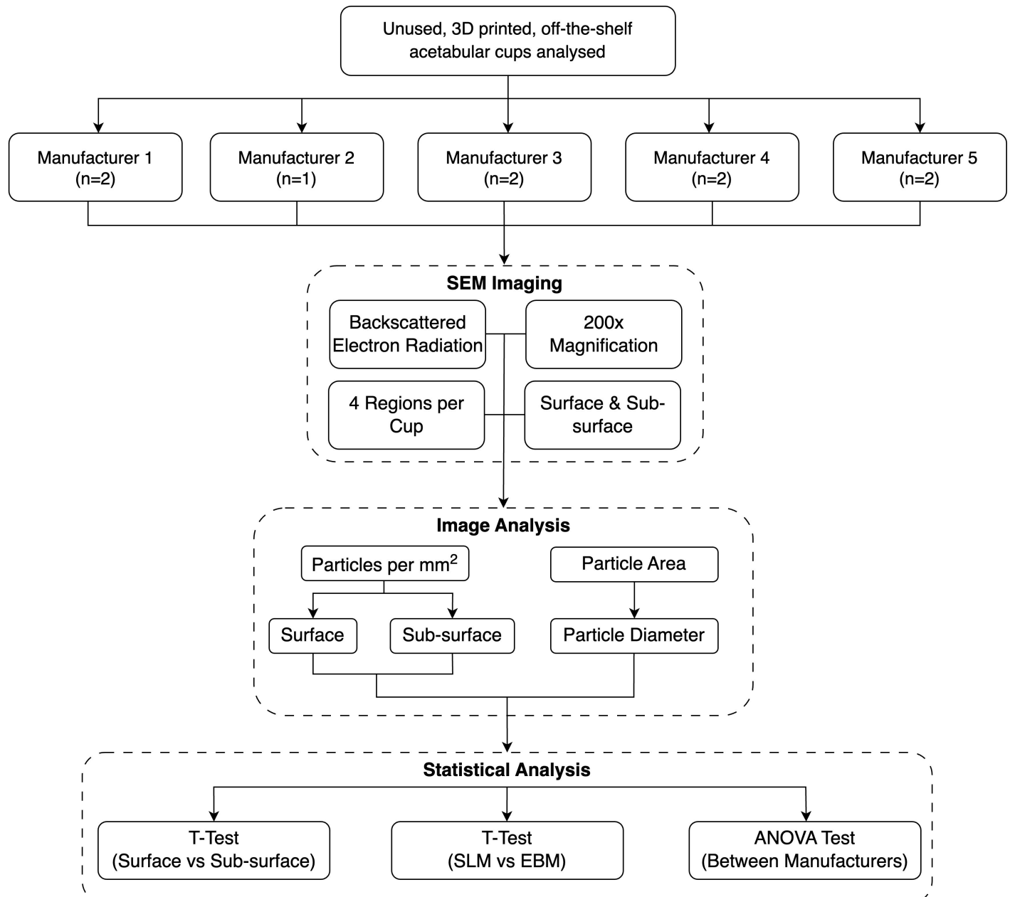
Figure 4.01: The study design showing the analysis steps that were performed on unused, 3D-printed, off-the-shelf implants that were obtained and imaged using backscattered electron radiation scanning electron microscopy, where the particle diameter and particles per mm 2 were calculated using ImageJ, followed by suitable statistical analysis [125].
