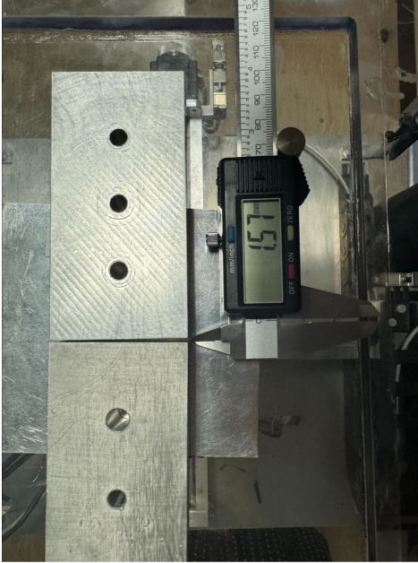
Fig. 12. Photo of the taper gap between two aluminium plates placed close together. Each plate has a 100.0 mm length, 50.0 mm width and 20.0 mm thickness. A taper gap is generated from the left-hand side to the right-hand side with a maximum gap width of 1.57 mm. The structure is shielded by a 0.42 mm aluminium sheet with an additional 1.50 mm rubber sheet between the two block structure and the aluminium sheet.
