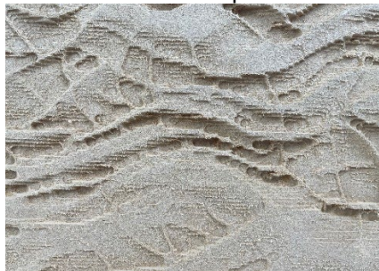
Figure 1. Concrete, cork and moss hybrid. CNC model for casting mold. Source: John Herrera, 2024.
