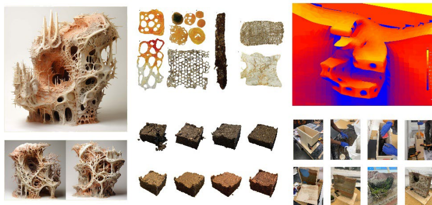
Figure 3. Chitosan / rammed earth hybrid structure: Explorations in Midjourney, material experiments, physical prototyping and Ladybug simulation. Source: Naqib Nasser, 2024.
