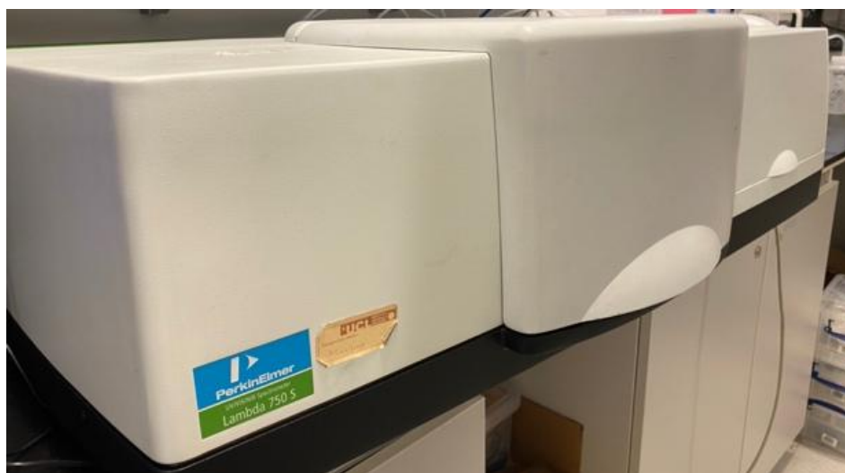
Figure 2.7: The Perkin Elmer Lambda 750S instrument used for UV-Vis measurements.
