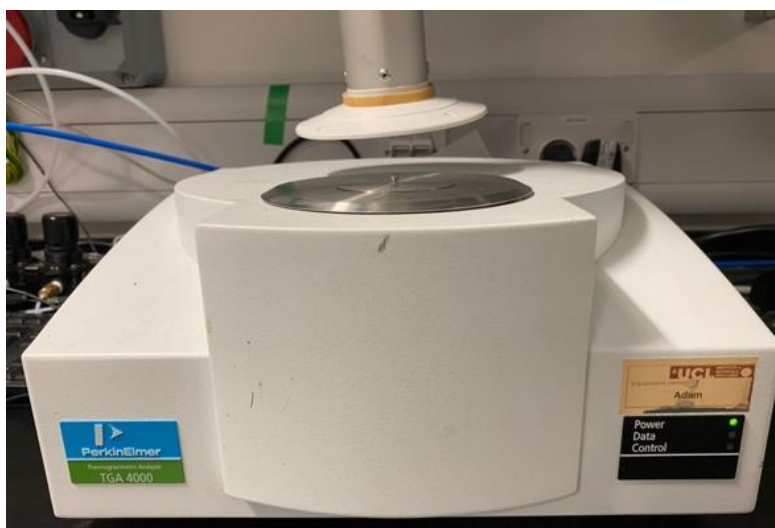
Figure 2.8: Physical instrument PerkinElmer TGA 4000 used for TGA measurements.
