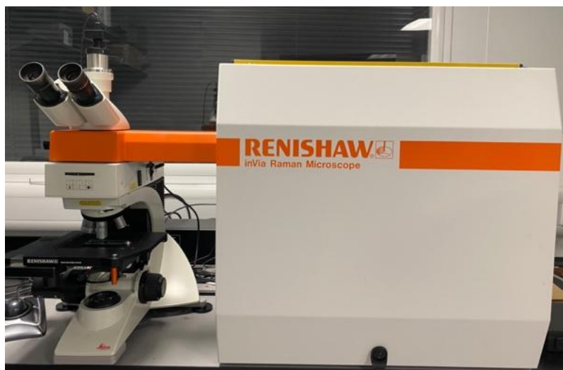
Figure 2.5: The Renishaw inVia™ confocal Raman microscope used to get Raman spectroscopy measurements.
