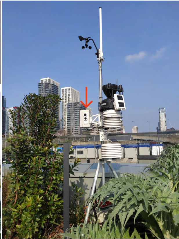
Figure 5.4: Deployment of acoupi devices at the People and Nature Lab Garden (A) Sensing Unit Components: single-board computer (Raspberry Pi 4B) and ultrasonic microphone (Dodotronic Ultramic 250k). (B) Protective Enclosure: housing two SBCs, one running acoupi_batdetect2 and the other acoupi_birdnet . (C) Field Deployment: enclosure mounted alongside other environmental sensors at the UCL East campus, Stratford, London.
