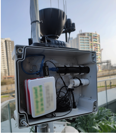
Figure 5.4: Deployment of acoupi devices at the People and Nature Lab Garden (A) Sensing Unit Components: single-board computer (Raspberry Pi 4B) and ultrasonic microphone (Dodotronic Ultramic 250k). (B) Protective Enclosure: housing two SBCs, one running acoupi_batdetect2 and the other acoupi_birdnet . (C) Field Deployment: enclosure mounted alongside other environmental sensors at the UCL East campus, Stratford, London.
