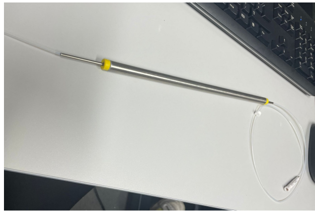
Figure 4.8: Mock endoscope fabricated for use in conjunction with OpUS probe.
