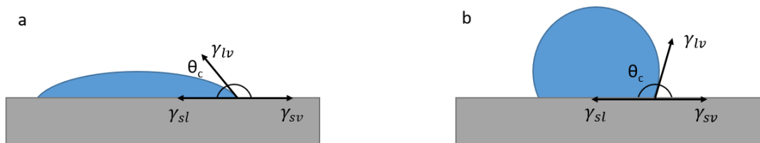
Figure 21: Differing wettability's of droplets on different surfaces. A droplet on (a) a high energy surface and (b) a low energy surface.
