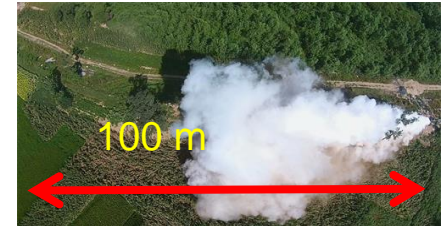
Release of 3.8 tons of Supercritical CO 2 from a large-scale pipeline (DUT, CO 2 QUEST)
