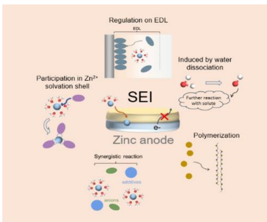
Figure 1.19 Illustration of the structure and functions of SEI on zinc anodes. Reprinted with permission from ref. [212] Copyright 2023 Wiley-VCH GmbH.
