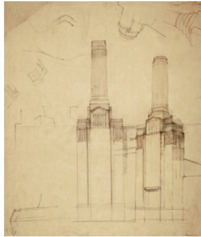
421. Battersea Power Station, sketch by Scott for chimney tower designs with segmental pediments, c.1930-1
