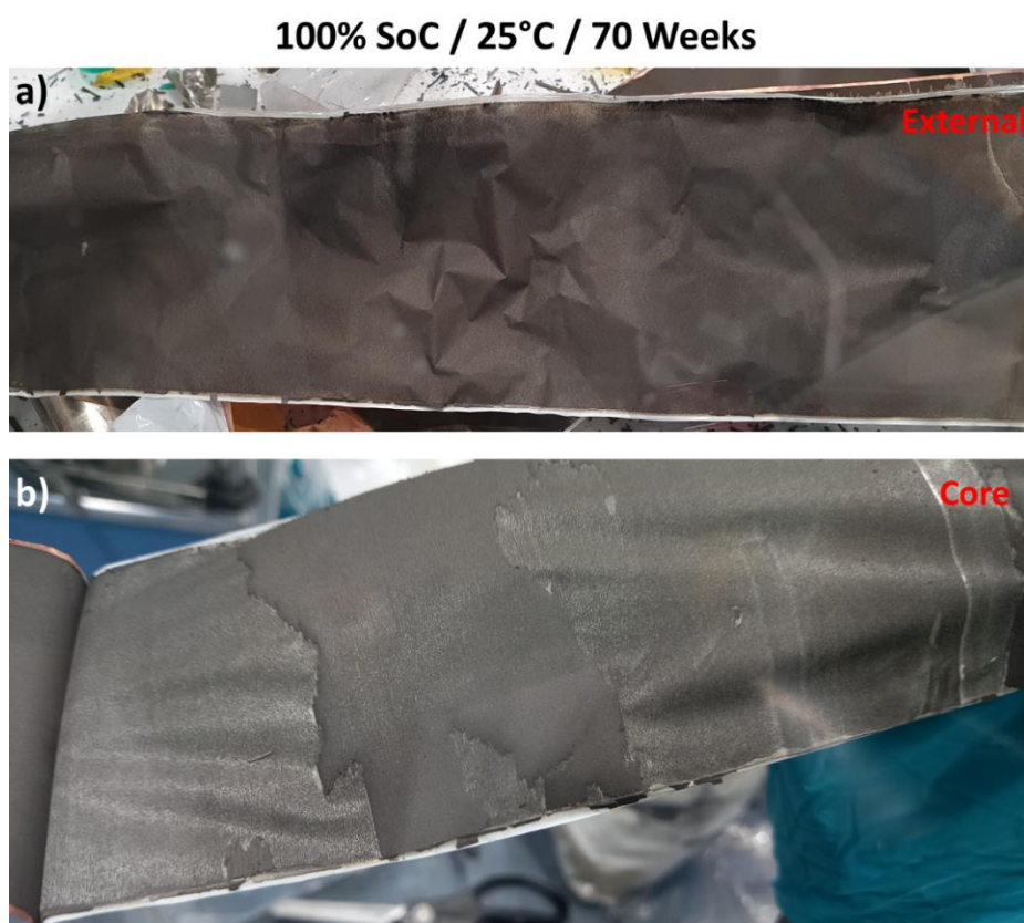
Figure 6-8. Photographs of anode side of the separator from a cell stored at 100% SoC, from the 25°C and 70 weeks batch, with distinction between areas at the outside and close to the core of the jelly-roll.
