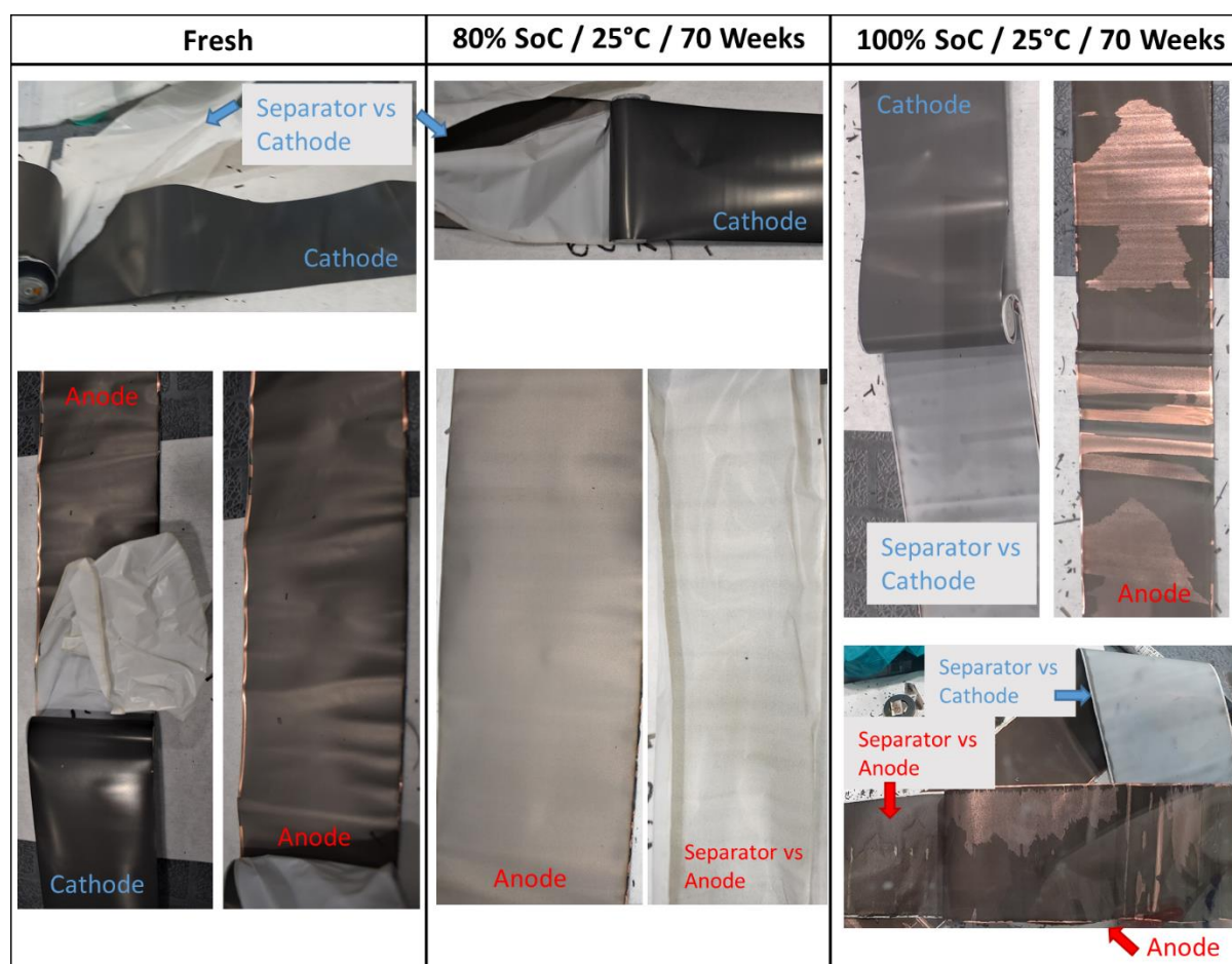
Figure 6-7. Photographs of the disassembled cylindrical cells, at a) fresh, b) 80% SoC and c) 100% SoC, from the 25 °C and 70 weeks batch. Particular attention is brought to the state of the cathode, anode and their corresponding side of the separator.
