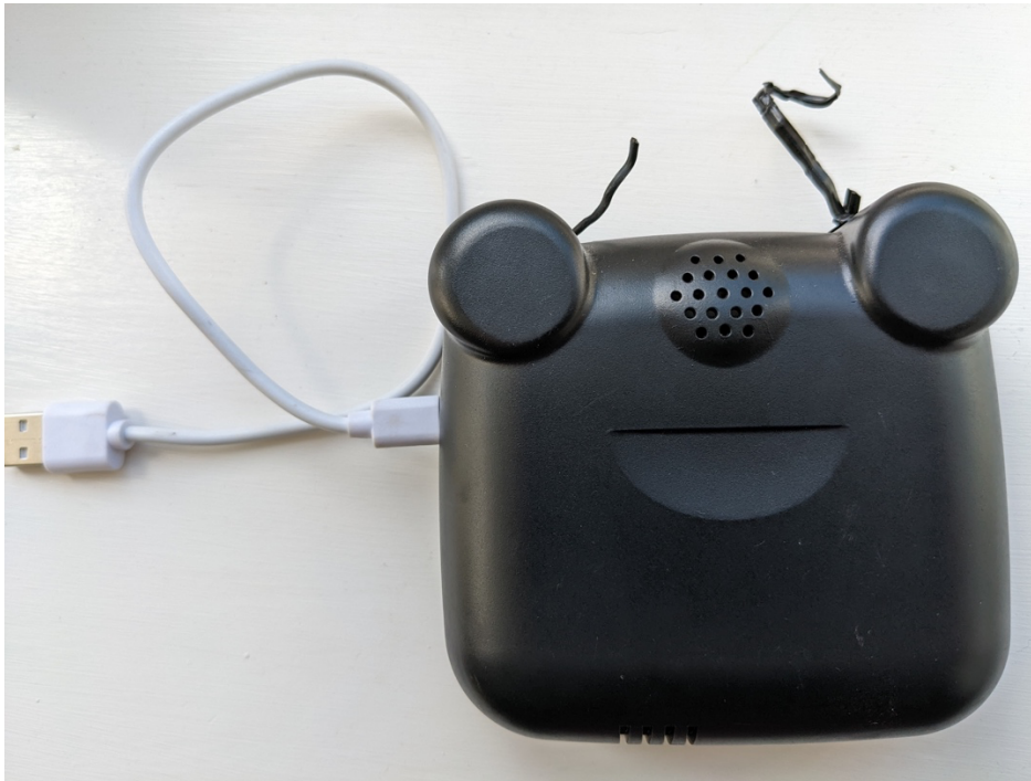
Figure 20. AirBeam machine to measure particulate matter in the air.
