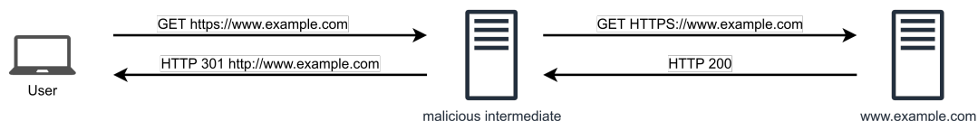
Figure 2.5: A simple representation of an SSL Stripping Attack. In this setup, the user initially requests a HTTPS connection, the malicious server intercepts this request and does not reply to the user. Assuming the website does not support HTTPS, the user’s browser automatically then makes an insecure HTTP request which is fulfilled by the malicious server.
