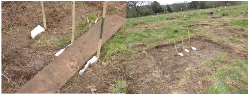
Figure 4 • Measuring out and inserting CSA cotton strips and marking with short bamboo poles for later retrieval. Left: into a Scarified plot. Right: into a Deturfed plot. 12 March 2021.
