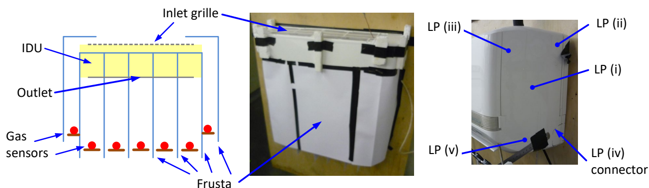
Figure 1: Diagram and photographs of the test arrangement: construction of the frusta and sampling points (left), photograph of the frusta (centre) and selected leak positions (LP) within the IDU right end.
