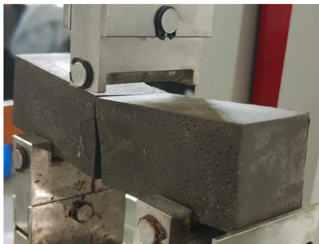
Figure 4.6. Failure pattern of AAFS paste after three point-bending tests.
