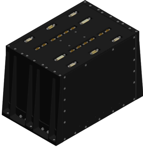
(a) The ICU box mechanical drawing.
