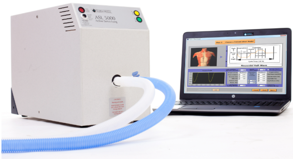
Figure 5.4.: ASL 5000 Lung Simulator used to replicate adult breathing patterns at various physiological parameters
