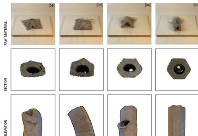
10 Relation of the clay moisture and needed air pressure for extrusion.
