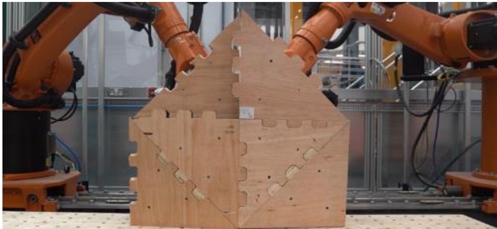
Figure 1 Multi-Robotic Assembly of Timber Plate Structures
