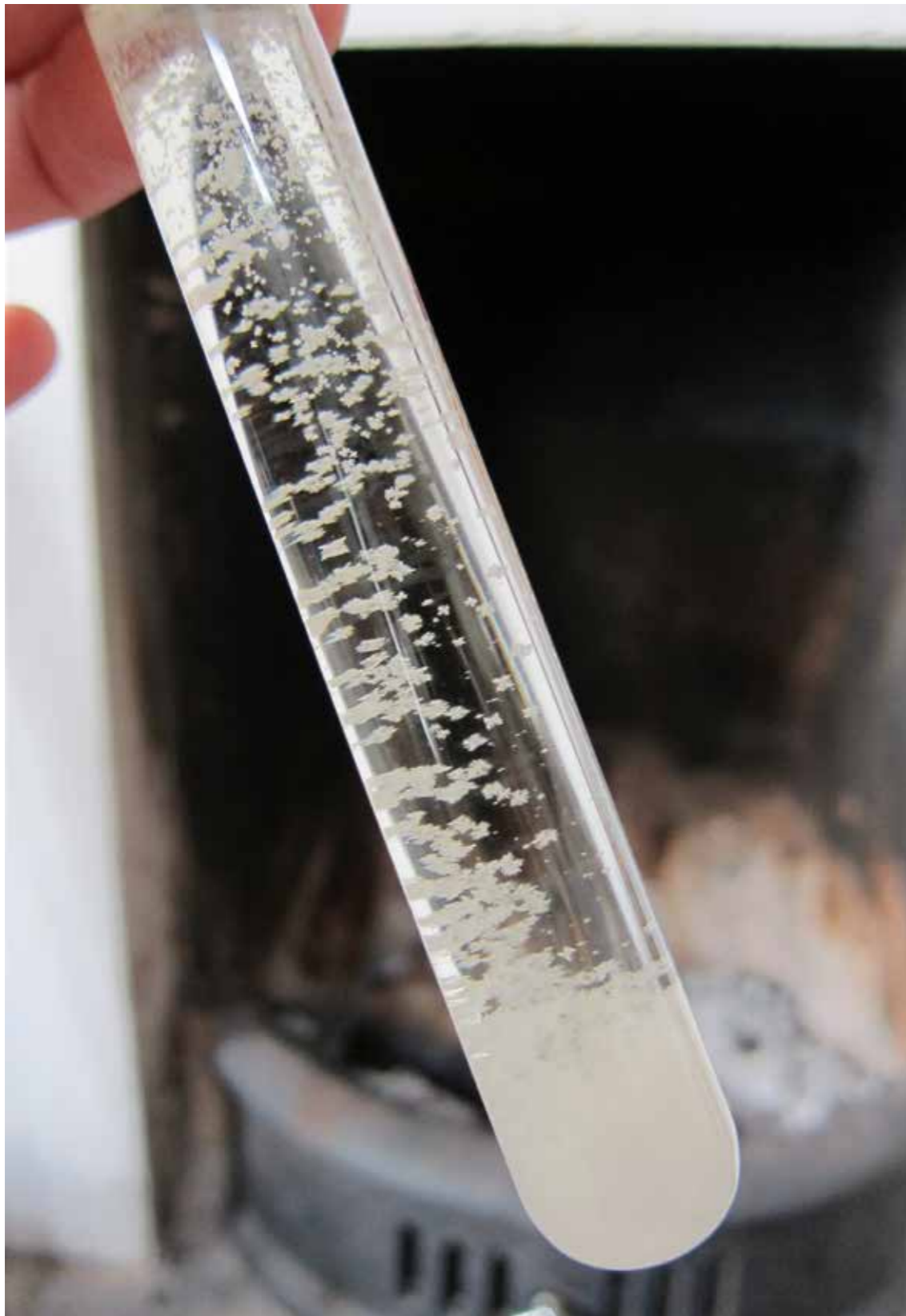
Saturated camphor solution crystallising with weather conditions for use in the Liminal Organs barometers. Appendix A p.32
