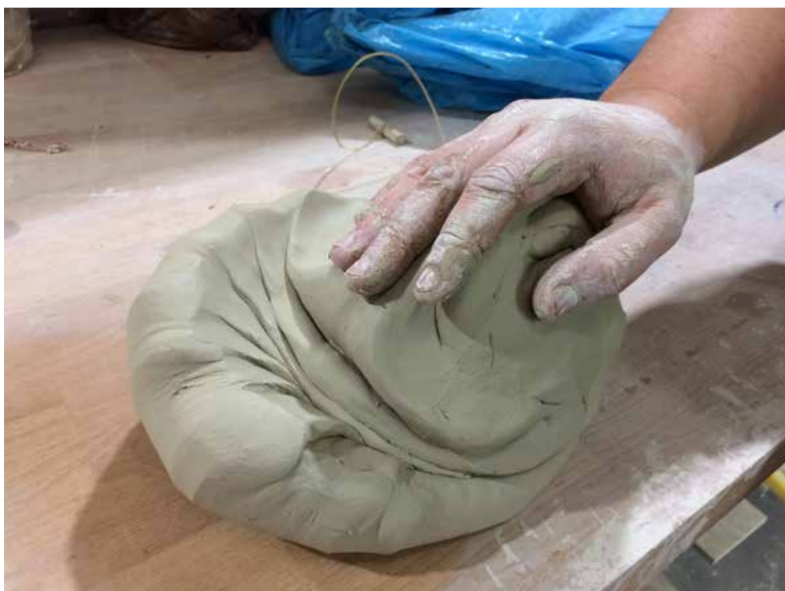
Spiral clay mixing technique which aligns the microscopic internal flat particles of clay so that when that clay is thrown on the wheel - also a spiral motion - the resulting object is less likely to warp or crack when it shrinks as it dries and is fired in the kiln. Potter: Darren Ellis.
