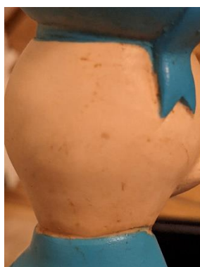
Figure 84: The dirtied surface of sample DOD. The surface was cleaned effectively (top left area) by localised application of a cotton swab wetted with isopropanol: water mixture (50%)
