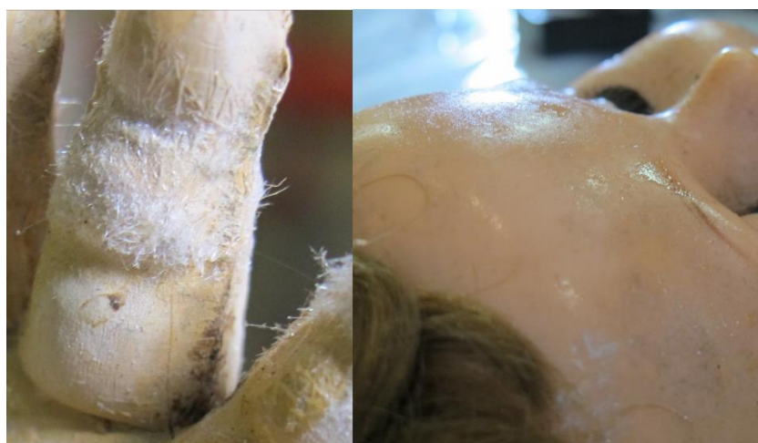
Figure 4: (Left) Bloom of triphenyl phosphate plasticiser and (right) phthalate plasticiser exudation from dolls made of cellulose acetate. Images are reproduced with the permission of Tate, London. Both dolls form a part of 'Mouth Open, Teeth Showing (I)', 2000, Zoe Leonard, Tate X717743 L04293.
