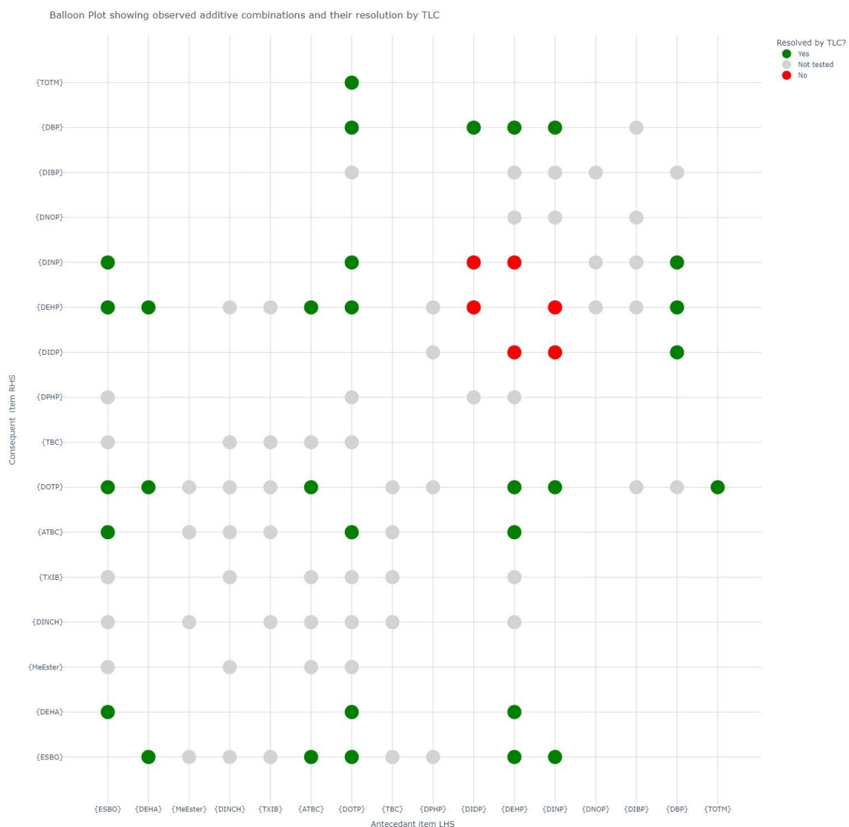
Figure 90: Scatter plot showing all plasticiser combinations observed in the literature dataset, colours indicate if the combination has been tested by TLC and can be resolved (green), cannot be resolved (red) or have not been tested (grey) using the proposed TLC method.
