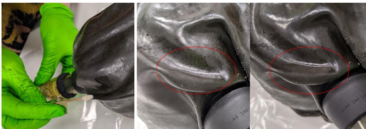
Figure 82: Swab cleaning of AmbuBag surface, showing controlled application with a microemulsion solution (left) before cleaning with ethanol/water mix (centre) and after with dull and tide-marked surface (right).
