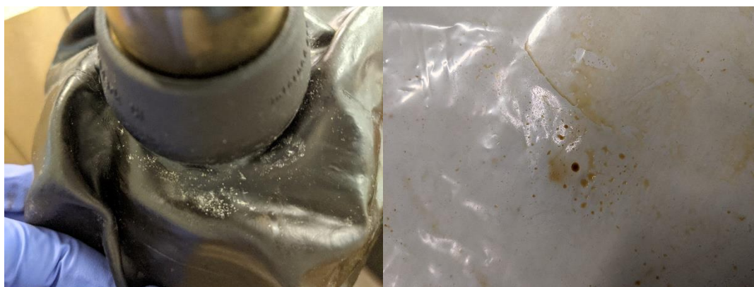
Figure 81: An 'AmbuBag' bag valve mask exhibit (RCA/UCL Culture), with bloom (left) and orange liquid on polyethene bag wrapper (right).
