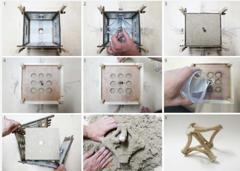
▲ Figure 1 Fabrication Process // GAD RC6 / Team SanDPrint: Xlyanzi Cao, Shuo Liu & Zeyn Yang
