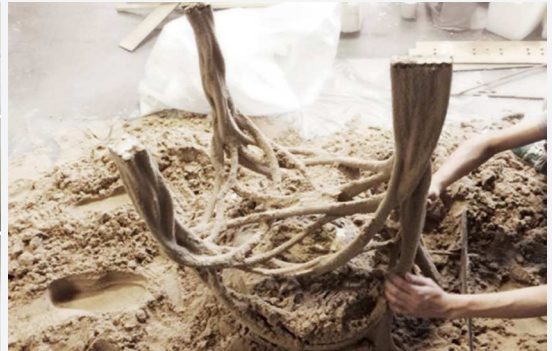
▲ Figure 2 Process of removing the casted piece from the sand mould // GAD RC6 / Team SanDPrint: Xlyanzi Cao, Shuo Liu & Zeyn Yang
