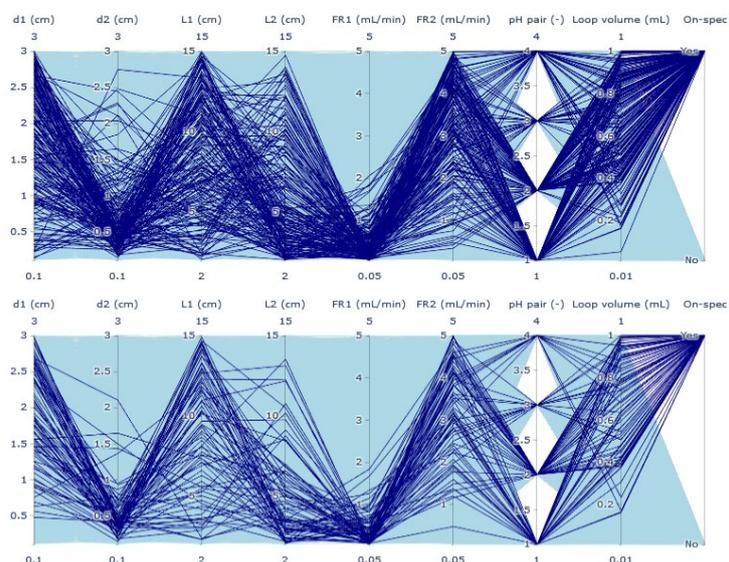
Figure 1. Parallel plots of the different scenarios tested for the 8-component mixture (top) and 16-component mixture (bottom). The dark blue lines refers to the feasible (on-spec) designs.
