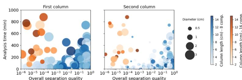
Figure 2. Bubble plot of the overall separation quality vs. analysis time of on-spec designs. The bubble size and color gradient refer to column internal diameter and column length, respectively, for the 1D column (left) and 2D column (right). The blue and orange color-maps refer to the 8-component and 16-component mixtures, respectively.
