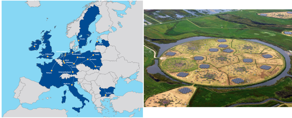
Figure 4.5: Left map: The current map of international LOFAR telescopes AST (2024) . Right photo: Aerial photo of the Superterp, the heart of the LOFAR core. There are groups of big black blocks laying in arrays in the photo, these are high-band antennas (HBAs), and the small blocks are low-band antennas (LBAs). van Haarlem et al. (2013)
