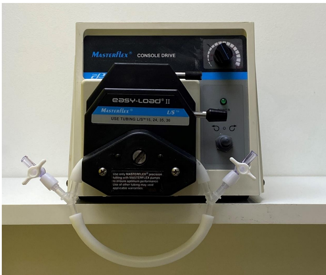
Figure 4-2 Picture of the closed-loop peristaltic pump device clamped in place in a peristaltic pump.
