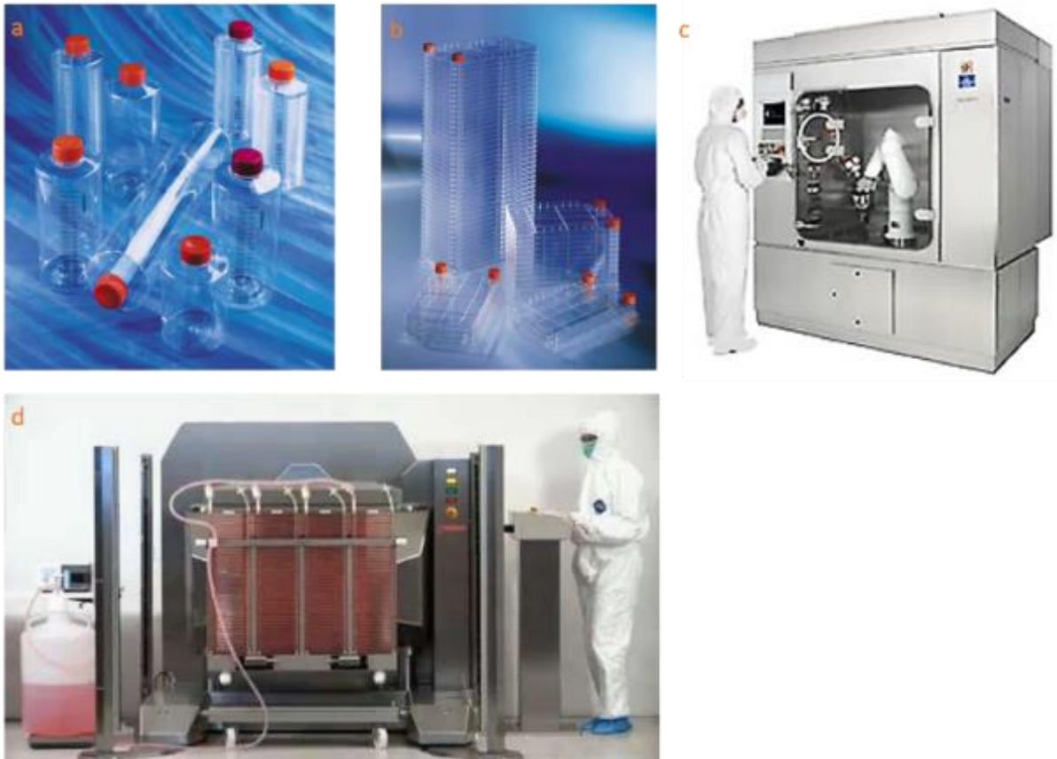
Figure 1.3: Static culture devices for adherent cell viral vaccine production. (a) Roller bottles with standard or expanded surfaces and a number of different surface areas; pictured are Corning® Roller Bottles (Corning, n.d.). (b) Multi-tray system consisting of a series of stacked trays; pictured are Corning® CellSTACK® cell culture chambers (Corning, n.d.). (c) Automated roller bottle processing; pictured is Cellmate automated cell culture system from TAP Biosystems (TAP Biosystems, n.d.). (d) Automated multi-tray units processing; pictured is Nunc™ automatic cell factory manipulator (Thermo Scientific, n.d.).
