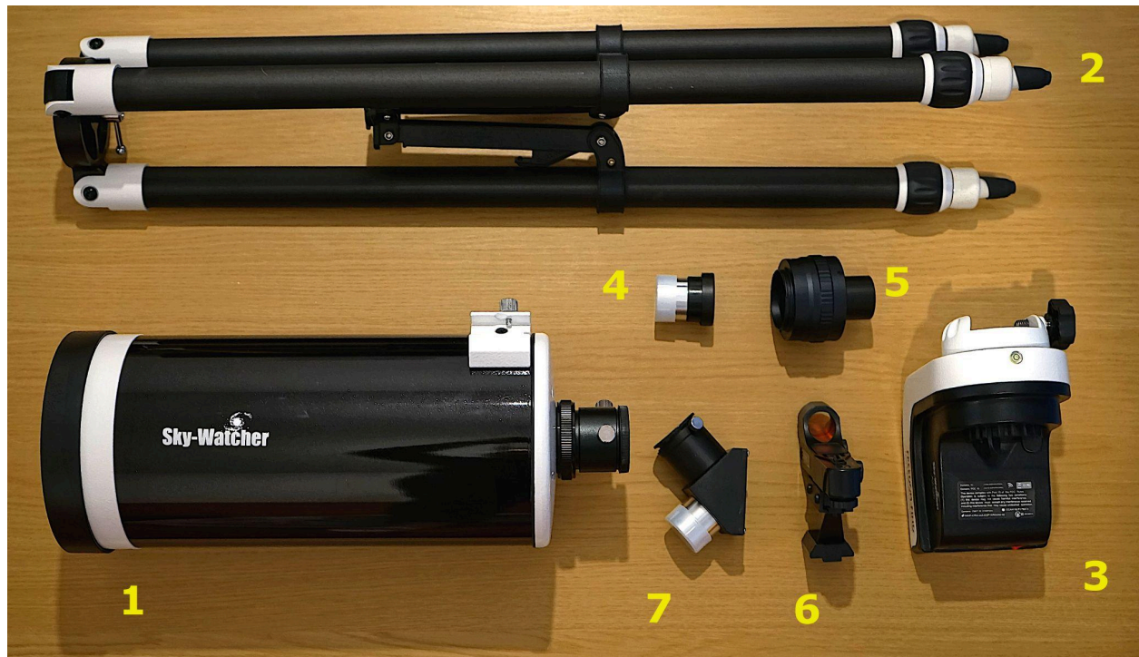
Fig. 9: The Anatomy of a Telescope. My telescope, broken down into its constituent parts, which are 1) the barrel, 2) the tripod, 3) the mount, 4) the eyepiece, 5) the T-ring for replacing the eyepiece with cameras, 6) the finderscope, and 7) the diagonal prism.
