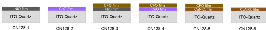
Figure 125. Illustration depicting the deposition process CuO, NiO, CFO-NiO, CFO-CuO, CFO-CuNiO x and CuNiO x films on ITO-quartz substrate
