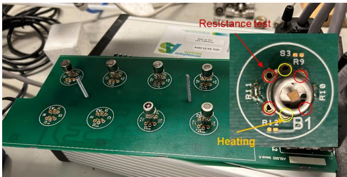
Figure 31. Digital image of gas sensors inserted into circuit board in the gas sensing box
