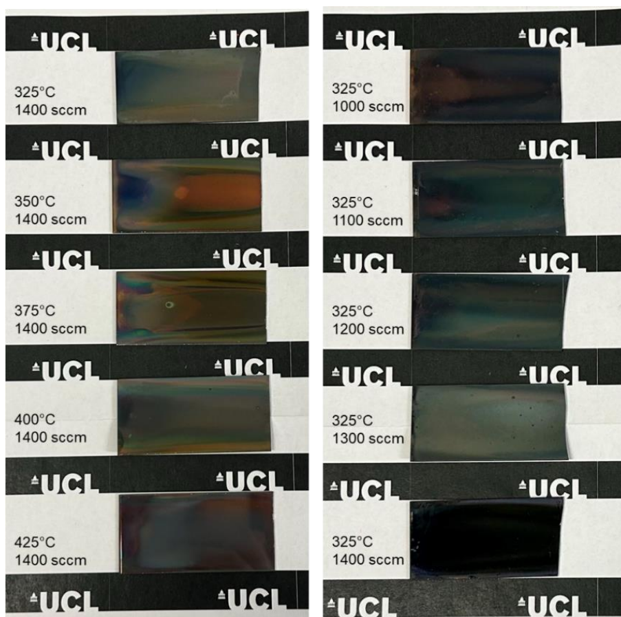
Figure 49. Digital photos of CFO-ACAC films: (Left) deposited at five different temperatures ranging from 325°C to 425°C, with gas flow rate of 1000 sccm to 1400 sccm and Cu/Fe precursor ratio of 0.15 mmol/0.15 mmol; (Right) deposited at 325°C with five different flow rates ranging from 1000 sccm to 1400 sccm, Cu/Fe precursor ratio of 0.15 mmol/0.15 mmol
