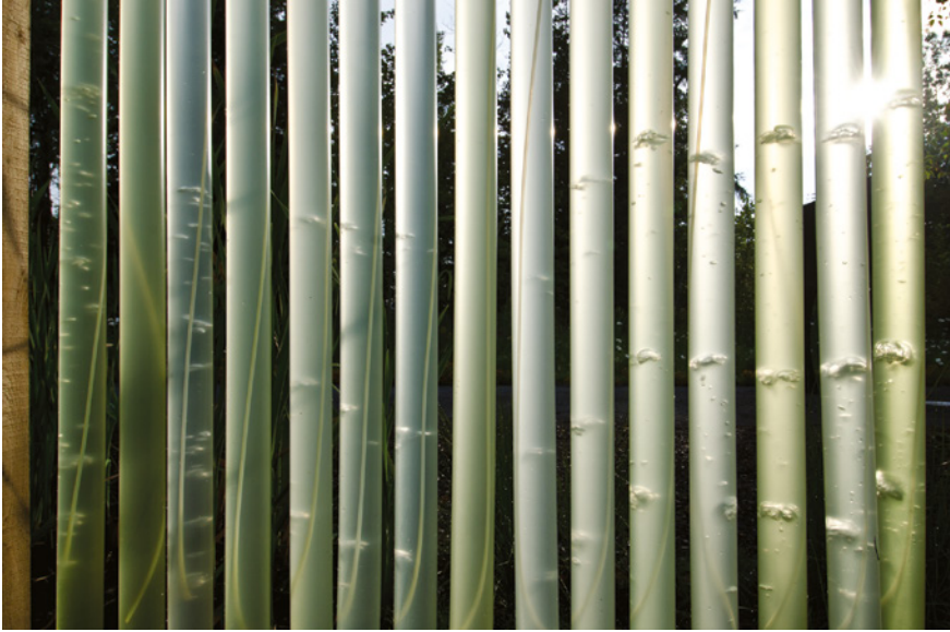
FIGURE 11.4 Algaegarden – detail of bioreactor tubes containing Chlorella cultures PHOTO CREDIT: LOUISE TANGUAY
