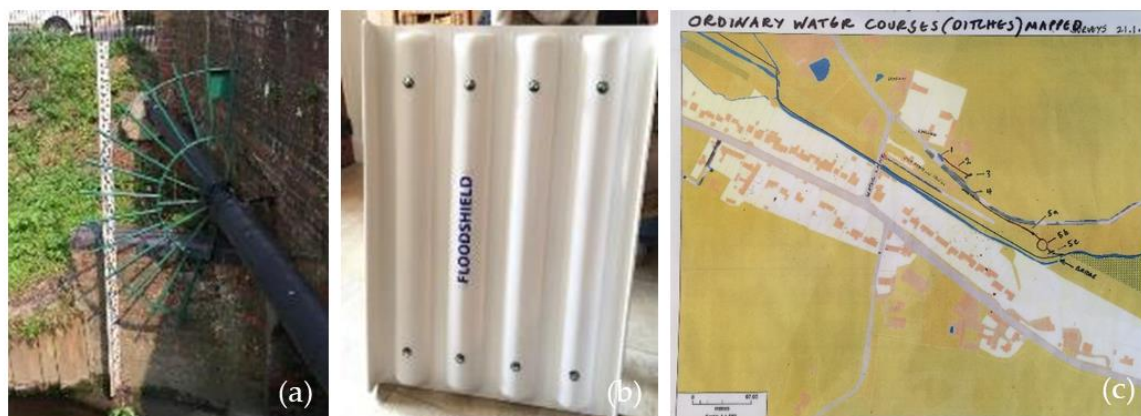
Figure 9. a) Flood depth gauge mounted in the stream across Sturmer by the residents, b) an example of a typical portable flood barrier owned by the residents, and c) ordinary water courses in Sturmer mapped by the Flood Action Group.
