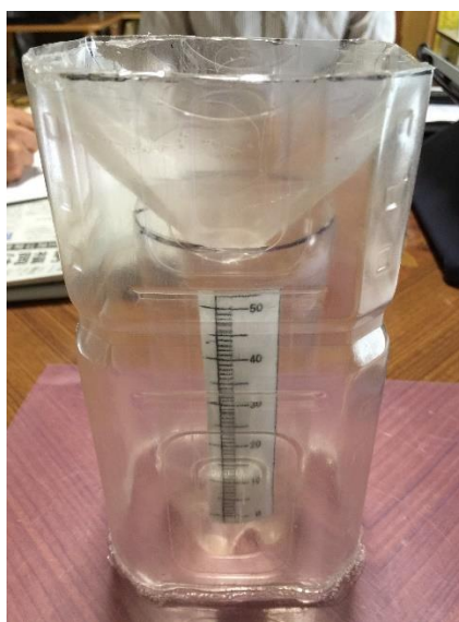
Figure 8 . A simple low-cost rain gauge produced by Jogucho community in Hita City as an early disaster preparedness strategy.
