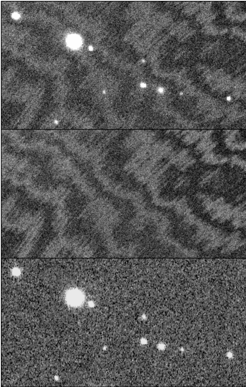
Figure 4.2: Three images showing the effect of fringing on the images on the Gemini-S i-band image of GRB 100316D. Top: raw image with fringing, middle: fringe frame image for subtraction, bottom: final fringing subtracted image.
