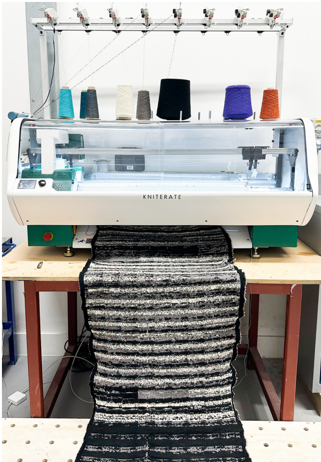
5 Fabrication of the textile with Kniterate.
