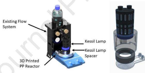
Figure 4: Proposed continuous flow photochemistry system designed to work seamlessly with existing Kessil lamps (depicted on the left). A detailed view (shown on the right) provides an illustration of the suggested lamp setup positioned above the 3D-printed reactor [57].
