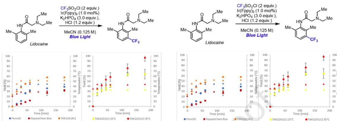
Figure 3: Performance comparison of two photocatalytic reactions across four different photoreactors and set-ups over time, monitoring the reaction yields (%) and reaction temperature (°C). [52]
