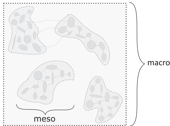
FIGURE 1 Schematic view of the multi-porous extension that considers a quasi-static medium at a macroscopic scale and distinguishes pore sets at a mesoscopic scale. Sets are allowed to be weakly connected (see upper part).
