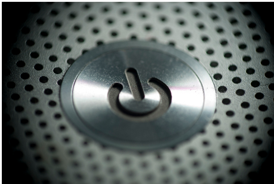
Figure 7. The Standby Symbol on a Macbook Pro Power Button. Photograph by vincentq, cc-by-sa-2.0. 28
