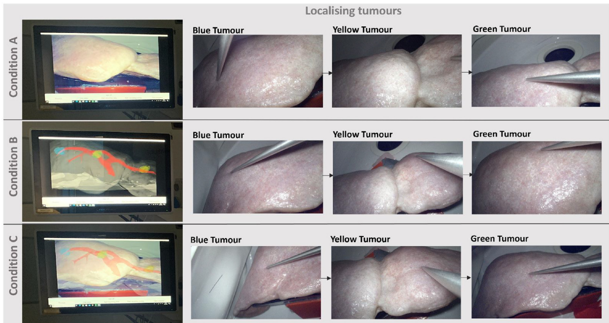
Fig. 3. Examples of Tumour localisation under three different conditions (Condition A: Baseline, Condition B: Split AR, and Condition C: Full AR). Smartliver AR system display (from the top left of Fig. 2) per condition is shown on the left, and each row shows the resulting ordered localisation attempt with the pointing instrument at the blue, yellow and green tumours. Note that the displayed view does not correspond to the view that the participant was experiencing at the moment of localising.
