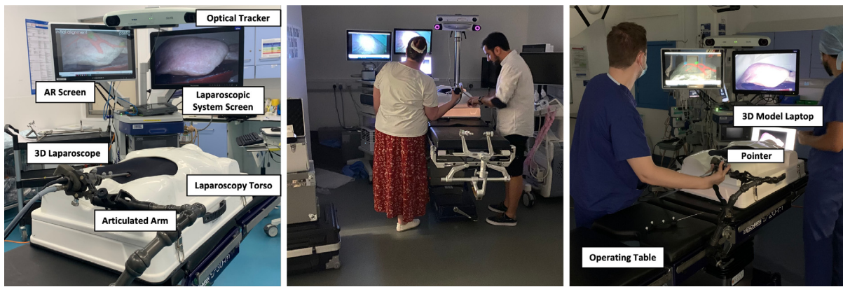
Fig. 1. Surgical simulation setup used in this study. Left: The setup used in operating theatres for surgeons. Middle: Example of engineering participant undertaking study in the mock operating room. Right: Example of surgeon participant undertaking study in hospital operating theatre.
