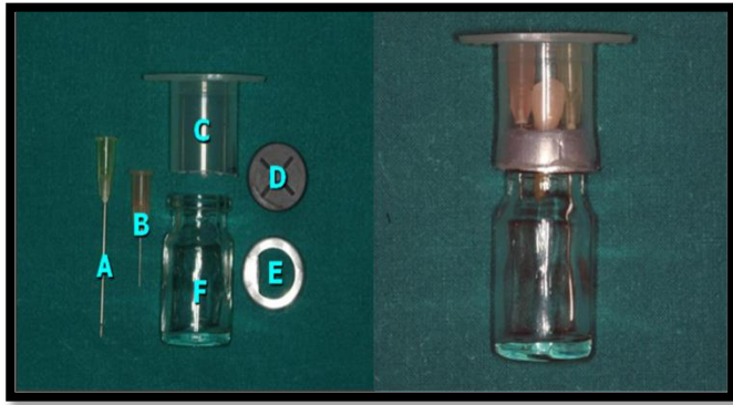
Figure 1. In vitro infection model A) 18G needle to replenish medium; B) 26G needle for ventilation; C) Sectioned 20 mL syringe; D) Rubber cap; E) Ring; F) 5 mL vial
