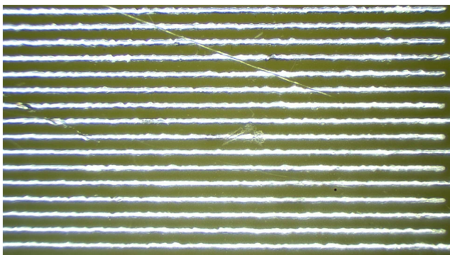
Fig. 7. Micrograph of bright surface on a solder coated Cu-FR4 interdigitated electrode with silicone encapsulation following aging. Imaged at 6.4\times magnification.
