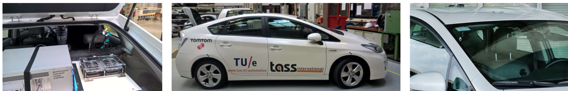
Fig. 6: A Toyota Prius autonomous driving research prototype vehicle equipped with Nvidia Drive PX 2, and Sekonix GMSL Camera. Sekonix GMSL Camera connected to Drive PX 2 over GMSL cable in a vehicle (center image). Drive PX 2 mounted in the trunk of a vehicle (left image). Sekonix GMSL camera which is mounted behind the front windshield, positioned close to the rear-view mirror (right image).
